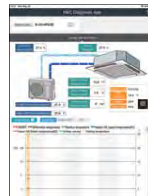
Refrigerant circuit view
