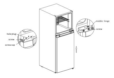
4) Remove the adjusting feet, lower hinge screw and lower hinge assembly, then install the lower hinge assembly on the other side of the box and install the adjusting feet on the side of the adjusting feet opening.
