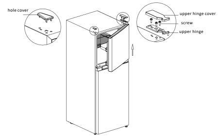
3) Unscrew the middle hinge screws, remove the middle hinge, and remove the two hole plug, a screw, a screw cap on the middle beam, then remove the refrigerator door.
