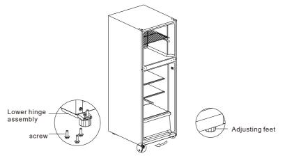
5) Dismantle the limit blocks and screws on the lower cover of both refrigerator door and freezer door, install them on the other side of both doors; then install the sleeve pipe on the upper cover of the refrigerator door on the other side.
