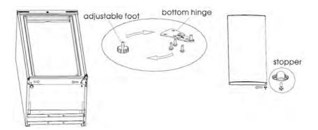
4) Assemble the shaft of the top hinge as in the picture below. Put the door on the bottom hinge, and assemble the upper hinge, upper hinge cover and the plastic screw hole cap successively.
