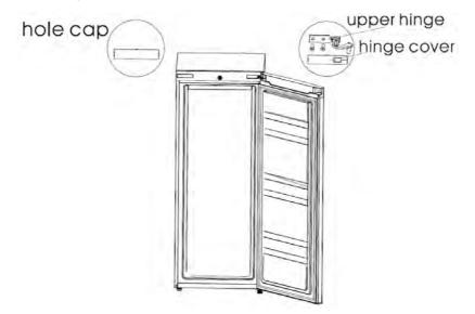
3) Remove the door and the bottom hinge assembly and the adjustable foot, then assemble the bottom hinge assembly and the adjustable foot on the other side. Remove the stopper from the right bottom side of the door, and assemble it on the other side of the door.
