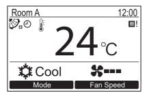
Clean the air filter when "⊞!" (filter sign) appears on the detailed display. (page 26)
