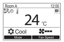
Reset the filter sign after cleaning the filter.
