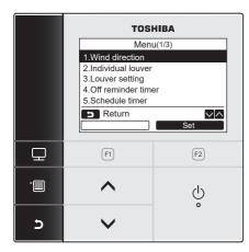
\* The menu screen returns to the normal / detailed display if no operation is performed for 60 seconds.
