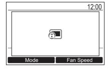
Details of operation lock activated by central control
